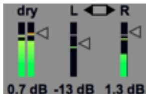
With these faders you can set the volume of the dry and wet signals. Please note that when the switch in the top between L and R is activated (pink) the faders are linked, while when the switch is off (gray) they are independent.
